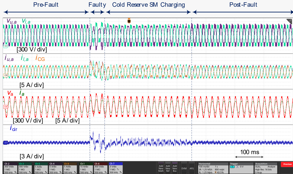
Experimental results during pre-fault, faulty, charging phase of cold reserve SM, and post-fault operation conditions:
